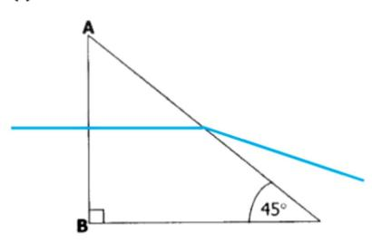
(iii) The critical angle (c) can be calculated using Snell's Law for the boundary between glass and air, which is:
